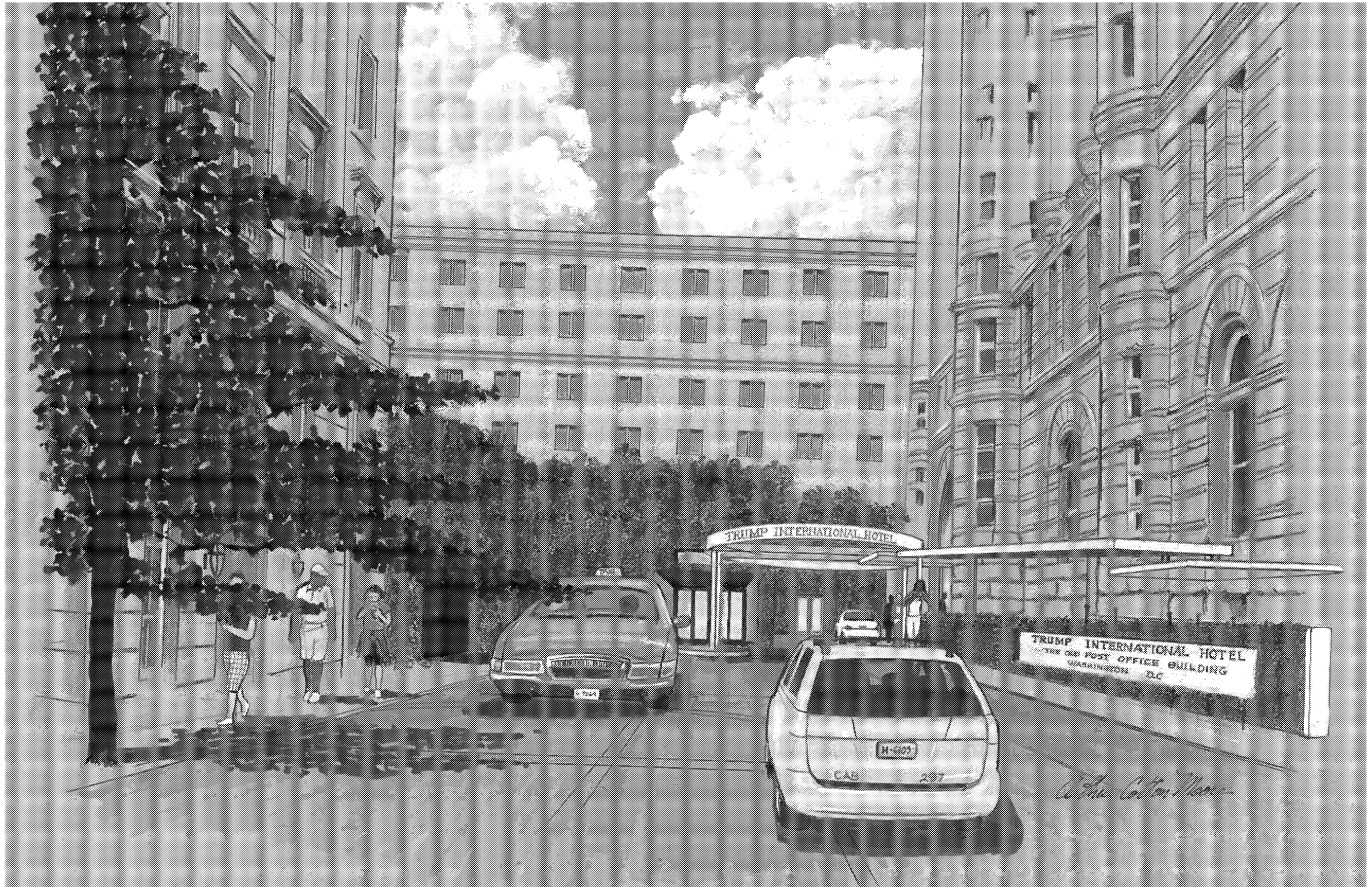
11th Street vehicular entry with Annex living green wall and glass canopy which is disconnected from the OPO.
