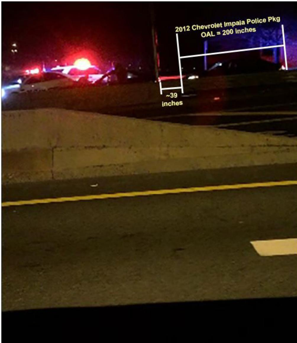
**Pixel Based Photogrammetry Based Upon CW-1 Cell
