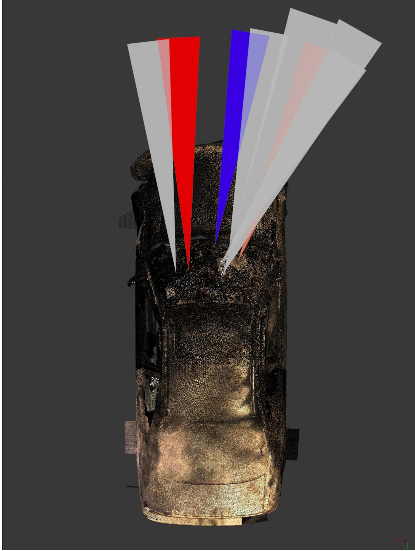
**3D Laser Scan Data of Honda Civic with Bullet Trajectory Cones**
