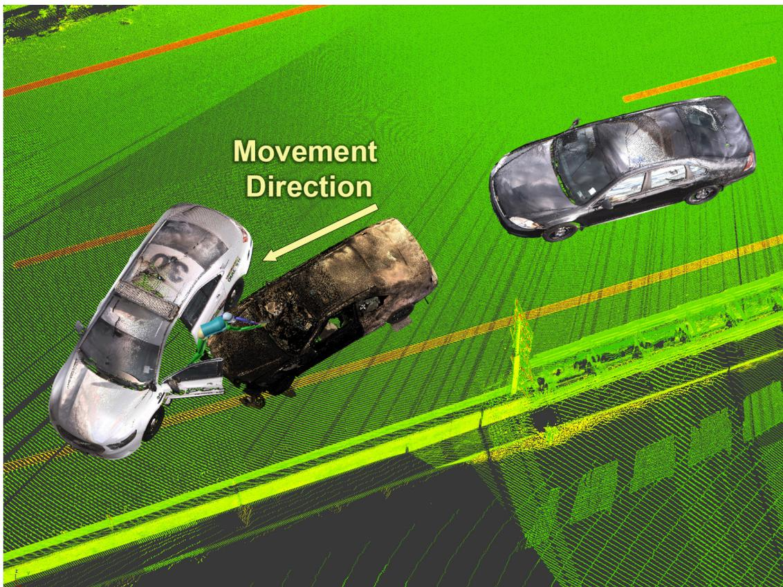
**Orientation of Honda and Sergeant French's Patrol Vehicle Doesn't Support a Relative Motion to the Left - Theoretical**
