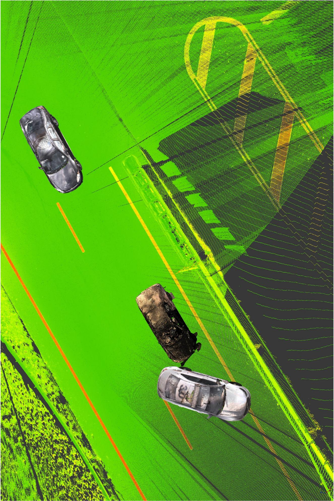
**Top Down View of 3D Working Model from PD Video Photogrammetry**
