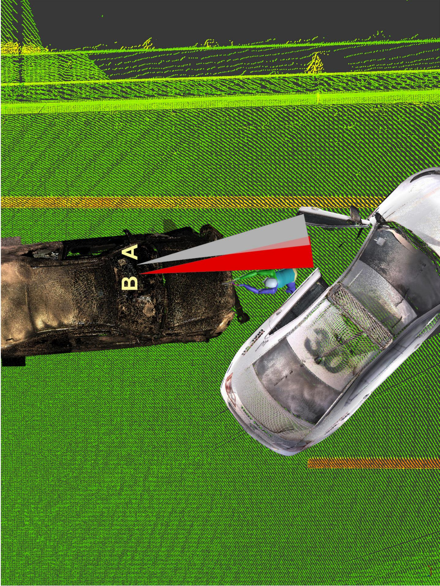
**Alignment of Trajectories A and B to Sergeant French's Position**
