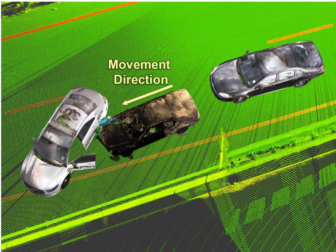
**Orientation of Honda and Sergeant French's Patrol Vehicle Doesn't Support a Relative Motion to the Left - Point of Rest**
