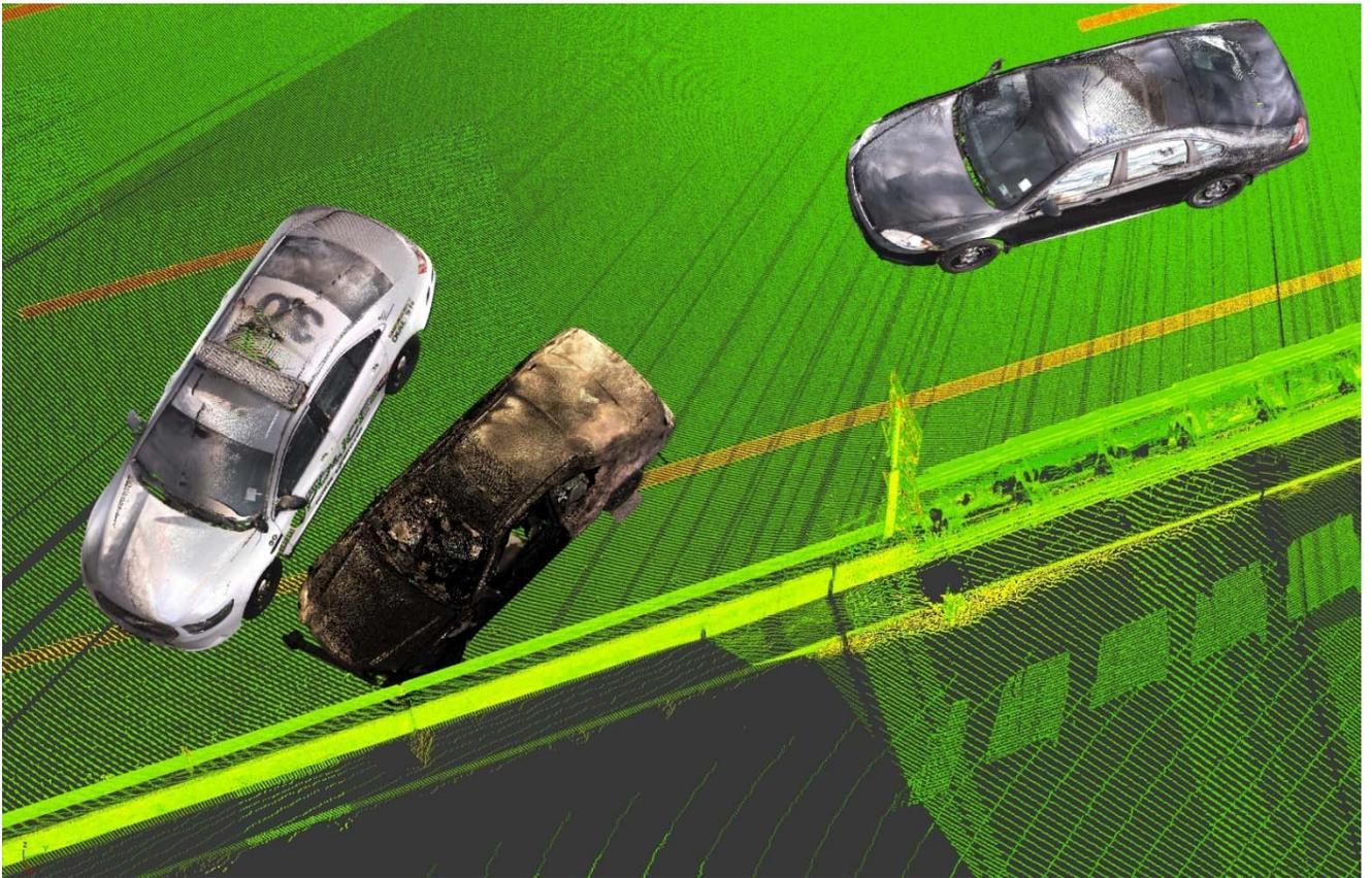
3. The rearward impact between the rear of the Honda and the front bumper area of the Impala. This impact is based upon the evidence of impact seen on the Honda passenger side rear bumper and matched to the damage pattern on the front bumper/grill area of the Impala as documented via 3D laser scan.
