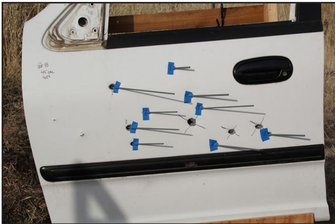
*Car Door with Ballistic Trajectory Rods*
