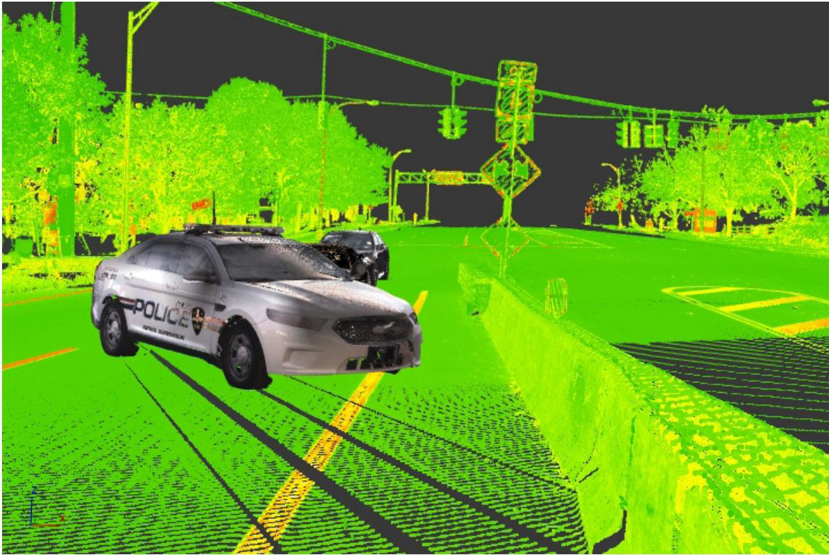
**3D Working Model from PD Video Photogrammetry**
