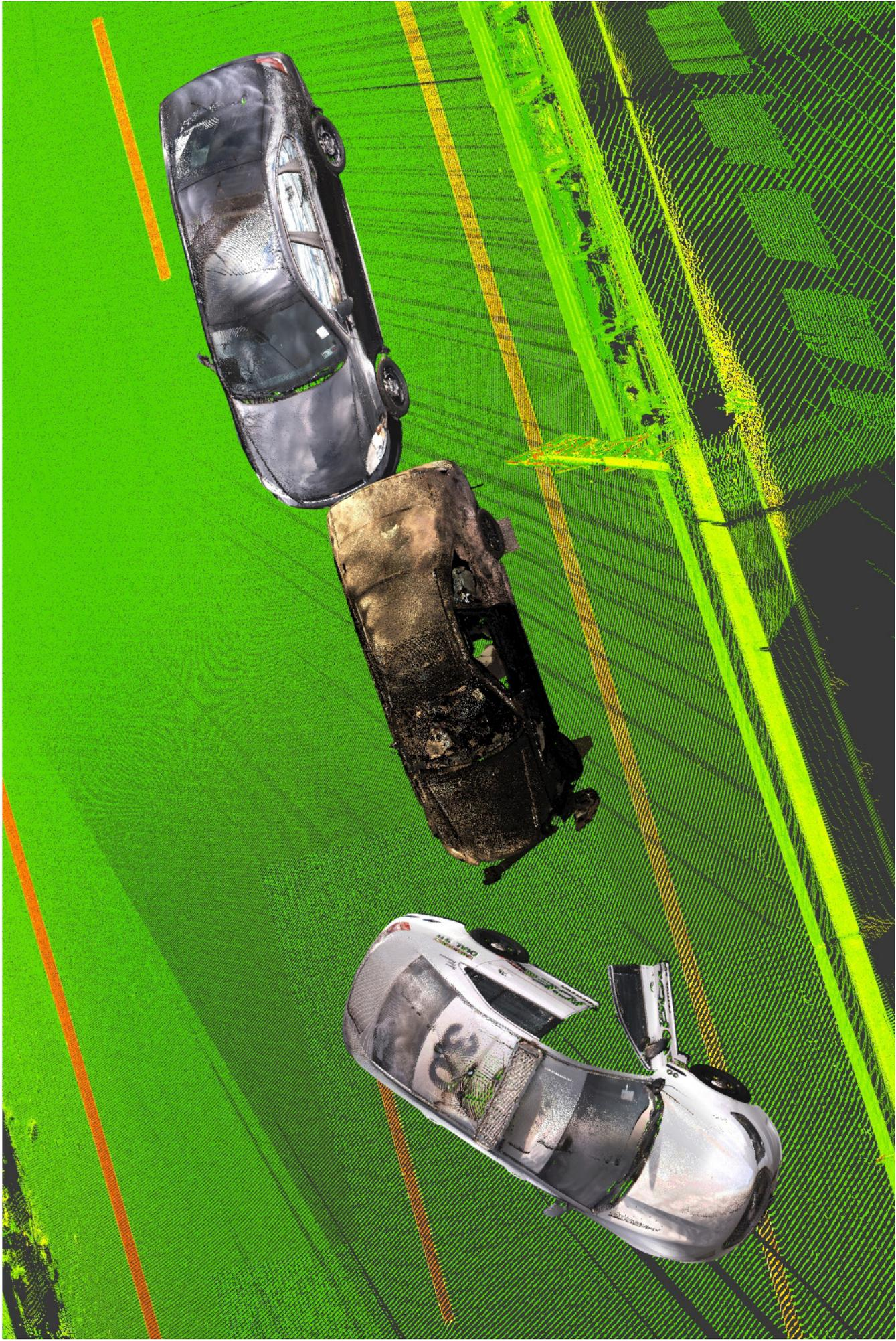
**Vehicle Kinematics for Honda in Reverse - Deepest Impact with Impala**
