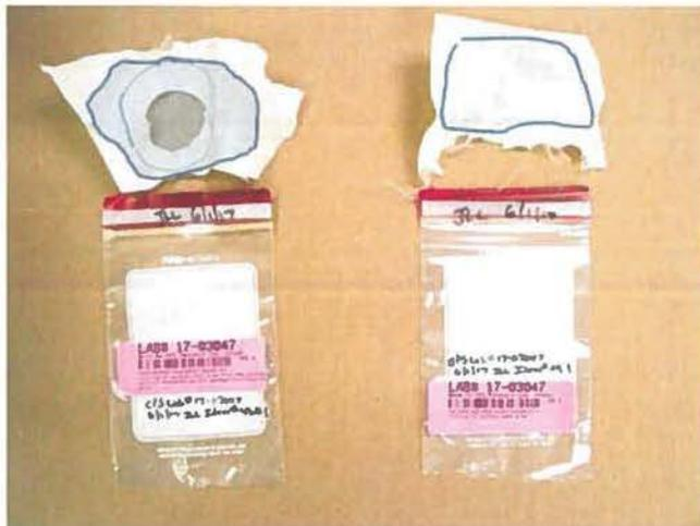
Prior to analysis, the tape lift stubs were carbon coated to a thickness of ~5 nm (~50Å) with the Gatan Model 681 coater in order to ensure electrical conductivity in the scanning electron microscope (SEM).
