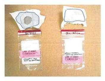
Prior to analysis, the tape lift stubs were carbon coated to a thickness of ~5 nm (~50Å) with the Gatan Model 681 coater in order to ensure electrical conductivity in the scanning electron microscope (SEM).
