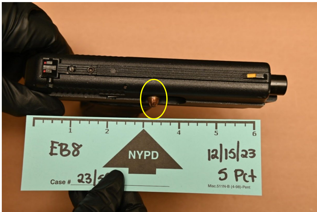
Crime Scene Unit photo of Mr. Edwards’s gun, showing bullet lodged in the slide’s ejection port.
